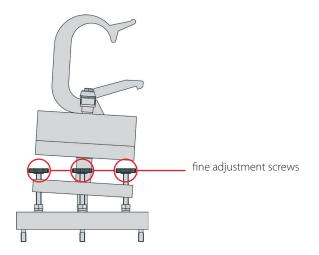
By means of the 4 adjustment screws, the positon of the truss mount can be defined very precisely.
