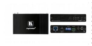
TP-583Txr is a high-performance, extended-reach HDBaseT transmitter for 4K HDR HDMI, RS-232 and IR signals over twisted pair. TP-583Txr converts all input signals into the transmitted HDBaseT signal. It enables extending video signal up to 100m (330ft) at 4K@60Hz (4:4:4) video resolution, up to 180m (590ft) at 4K@30Hz (4:4:4), and up to 200m (650ft) at HD video resolution over Kramer copper cables. It is compatible with standard HDBaseT-compliant extenders at 4K@30Hz and HD video resolutions
